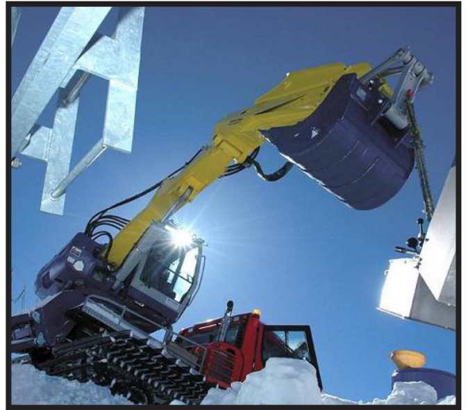
SYNTHETIC LOW TEMP UTF provides positive hydraulic control with oil operating temperatures from -76°F. (-60°C.)
